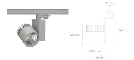
COB 3000 [K] CRI97 Light colour CRI Led chip flux 2601 [lm] Luminous flux 2080 [lm] System power 23 [W] Luminaire Efficiency 90 [lm/W] Beam angle 20° Controller ON/OFF MacAdam 3 SDCM
