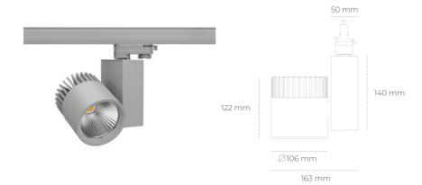
COB 3000 [K] CRI97 Light colour CRI 1144 [lm] Led chip flux Luminous flux 915 [lm] System power 10 [W] Luminaire Efficiency 92 [lm/W] Beam angle 20° Controller ON/OFF MacAdam 3 SDCM
