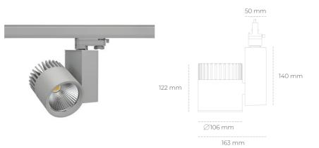
COB 3000 [K] CRI97 Light colour CRI 90 Led chip flux 1575 [lm] Luminous flux 1260 [lm] System power 14 [W] Luminaire Efficiency 90 [lm/W] Beam angle 15° Controller ON/OFF MacAdam 3 SDCM LUMINAIRE
