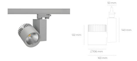
COB 3500 [K] PREMIUM WHITE Light colour CRI 90 Led chip flux 4038 [lm] Luminous flux 3230 [lm] System power 35 [W] Luminaire Efficiency 92 [lm/W] Beam angle 30° Controller ON/OFF MacAdam 3 SDCM
