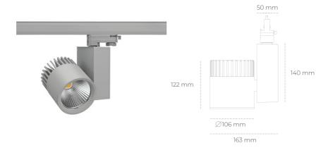
COB 3000 [K] PREMIUM WHITE Light colour CRI 90 Led chip flux 3911 [lm] Luminous flux 3128 [lm] System power 27 [W] Luminaire Efficiency 116 [lm/W] Beam angle 45° Controller ON/OFF MacAdam 3 SDCM
