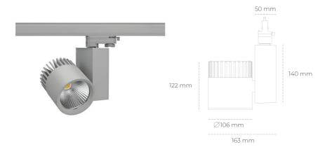
COB 3000 [K] PREMIUM WHITE Light colour CRI 90 Led chip flux 2064 [lm] Luminous flux 1651 [lm] System power 14 [W] Luminaire Efficiency 118 [lm/W] Beam angle 30° Controller ON/OFF MacAdam 3 SDCM
