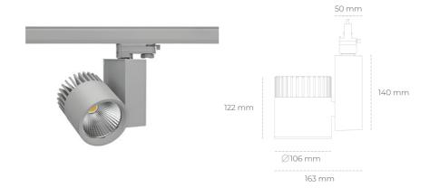
COB 5700 [K] SPECIAL Light colour CRI 3484 [lm] Led chip flux Luminous flux 2787 [lm] System power 27 [W] Luminaire Efficiency 103 [lm/W] Beam angle 20° Controller ON/OFF
