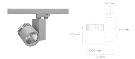
COB 5700 [K] SPECIAL Light colour CRI 4374 [lm] Led chip flux Luminous flux 3499 [lm] System power 35 [W] Luminaire Efficiency 100 [lm/W] Beam angle 15° Controller ON/OFF MacAdam 3 SDCM
