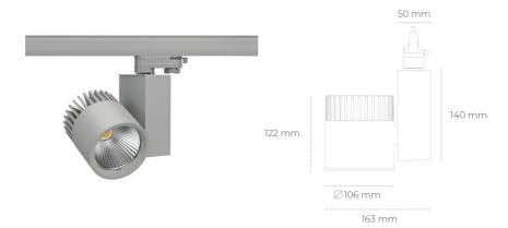
COB 4200 [K] MEAT WHITE Light colour CRI 90 Led chip flux 1412 [lm] Luminous flux 1129 [lm] System power 14 [W] Luminaire Efficiency 81 [lm/W] Beam angle 60° Controller ON/OFF MacAdam 3 SDCM
