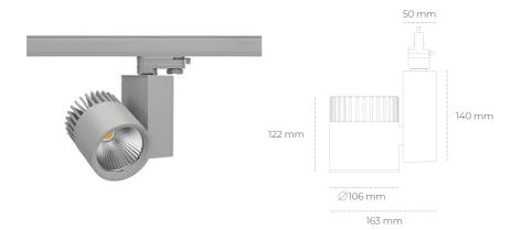
COB 4000 [K] HI EFFICIENT Light colour CRI 90 Led chip flux 1625 [lm] Luminous flux 1300 [lm] System power 10 [W] Luminaire Efficiency 130 [lm/W] Beam angle 45° Controller ON/OFF MacAdam 3 SDCM
