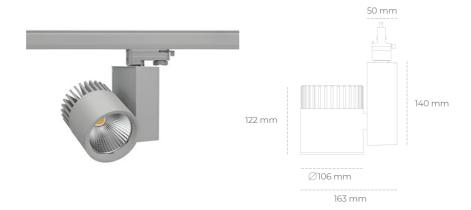
COB 4000 [K] HI EFFICIENT Light colour CRI 90 Led chip flux 3492 [lm] Luminous flux 2793 [lm] System power 21 [W] Luminaire Efficiency 133 [lm/W] Beam angle 15° Controller ON/OFF MacAdam 3 SDCM
