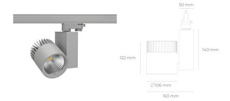
COB 3500 [K] HI EFFICIENT Light colour CRI 90 Led chip flux 4723 [lm] Luminous flux 3778 [lm] System power 31 [W] Luminaire Efficiency 122 [lm/W] Beam angle 60° Controller ON/OFF MacAdam 3 SDCM
