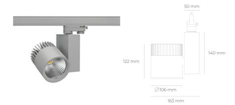
COB 3500 [K] HI EFFICIENT Light colour CRI 90 Led chip flux 3624 [lm] Luminous flux 2899 [lm] System power 23 [W] Luminaire Efficiency 126 [lm/W] Beam angle 60° Controller ON/OFF MacAdam 3 SDCM
