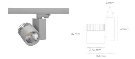
COB 3500 [K] HI EFFICIENT Light colour CRI 90 Led chip flux 5518 [lm] Luminous flux 4414 [lm] System power 36 [W] Luminaire Efficiency 123 [lm/W] Beam angle 45° Controller ON/OFF MacAdam 3 SDCM
