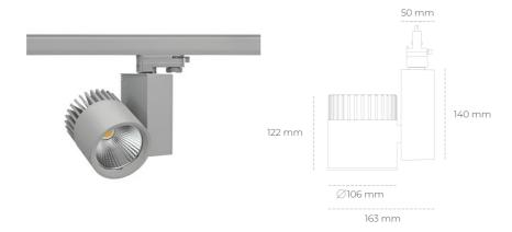
COB 3500 [K] HI EFFICIENT Light colour CRI 90 Led chip flux 4181 [lm] Luminous flux 3344 [lm] System power 27 [W] Luminaire Efficiency 124 [lm/W] Beam angle 45° Controller ON/OFF MacAdam 3 SDCM
