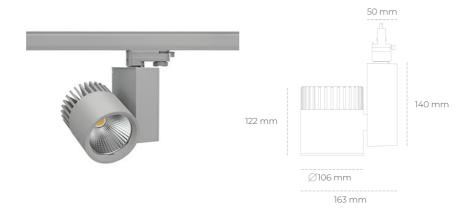
COB 3500 [K] HI EFFICIENT Light colour CRI 90 Led chip flux 5518 [lm] Luminous flux 4414 [lm] System power 36 [W] Luminaire Efficiency 123 [lm/W] Beam angle 30° Controller ON/OFF MacAdam 3 SDCM
