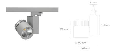
COB 3500 [K] HI EFFICIENT Light colour CRI 90 Led chip flux 4181 [lm] Luminous flux 3344 [lm] System power 27 [W] Luminaire Efficiency 124 [lm/W] Beam angle 30° Controller ON/OFF MacAdam 3 SDCM
