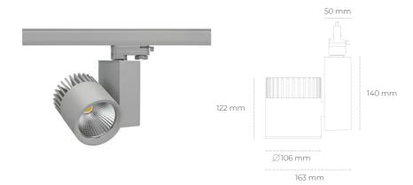
COB 3500 [K] HI EFFICIENT Light colour CRI 90 Led chip flux 5518 [lm] Luminous flux 4414 [lm] System power 36 [W] Luminaire Efficiency 123 [lm/W] Beam angle 20° Controller ON/OFF MacAdam 3 SDCM
