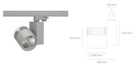
Track mounted LED spotlight. Aluminium housing. Ceiling base installation possible. Available in white, black and grey. Any RAL palette colour available on enquiry. Reflector beams available: 15°, 20°, 30°, 45° and 60°. Maximum power is 37W
