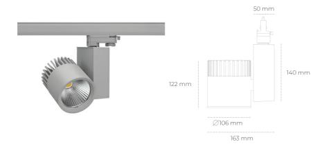
COB 3500 [K] HI EFFICIENT Light colour CRI 90 Led chip flux 1571 [lm] Luminous flux 1256 [lm] System power 10 [W] Luminaire Efficiency 126 [lm/W] Beam angle 20° Controller ON/OFF MacAdam 3 SDCM
