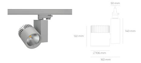
COB 3000 [K] HI EFFICIENT Light colour CRI 90 Led chip flux 3184 [lm] Luminous flux 2547 [lm] System power 19 [W] Luminaire Efficiency 134 [lm/W] Beam angle 45° Controller ON/OFF MacAdam 3 SDCM
