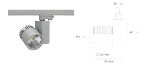
COB 3000 [K] HI EFFICIENT Light colour CRI 90 Led chip flux 1623 [lm] Luminous flux 1298 [lm] System power 10 [W] Luminaire Efficiency 130 [lm/W] Beam angle 15° Controller ON/OFF MacAdam 3 SDCM
