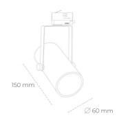
COB 3500 [K] HI EFFICIENT Light colour CRI 90 Led chip flux 2174 [lm] Luminous flux 1956 [lm] System power 14 [W] Luminaire Efficiency 140 [lm/W] Beam angle 15° Controller ON/OFF MacAdam
