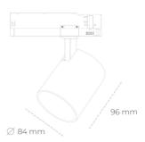
COB 3000 [K] HI EFFICIENT Light colour CRI 90 Led chip flux 3184 [lm] Luminous flux 2865 [lm] System power 19 [W] Luminaire Efficiency 151 [lm/W] Beam angle 15° Controller ON/OFF
