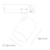
COB 3500 [K] HI EFFICIENT Light colour CRI 90 Led chip flux 3054 [lm] Luminous flux 2748 [lm] System power 19 [W] Luminaire Efficiency 145 [lm/W] Beam angle 23° Controller ON/OFF MacAdam 3 SDCM
