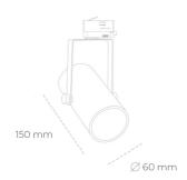
COB 3500 [K] HI EFFICIENT Light colour CRI 90 Led chip flux 1571 [lm] Luminous flux 1413 [lm] System power 10 [W] Luminaire Efficiency 141 [lm/W] Beam angle 38° Controller ON/OFF MacAdam 3 SDCM
