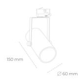
COB 3500 [K] HI EFFICIENT Light colour CRI 90 Led chip flux 4181 [lm] Luminous flux 3762 [lm] System power 27 [W] Luminaire Efficiency 139 [lm/W] Beam angle 23° Controller ON/OFF MacAdam 3 SDCM
