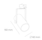
COB 2000 [K] MEAT PINK Light colour CRI Led chip flux 1741 [lm] Luminous flux 1566 [lm] System power 19 [W] Luminaire Efficiency 82 [lm/W] Beam angle 15° Controller ON/OFF
