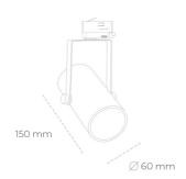
4200 [K] MEAT WHITE Light colour CRI 90 Led chip flux 2695 [lm] Luminous flux 2425 [lm] System power 27 [W] Luminaire Efficiency 90 [lm/W] Beam angle
