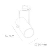
COB 4200 [K] MEAT WHITE Light colour CRI 90 Led chip flux 2159 [lm] Luminous flux 1943 [lm] System power 21 [W] Luminaire Efficiency 93 [lm/W] Beam angle 15° Controller ON/OFF MacAdam 3 SDCM
