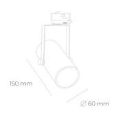
COB 4000 [K] HI EFFICIENT Light colour CRI 90 Led chip flux 4090 [lm] Luminous flux 3681 [lm] System power 25 [W] Luminaire Efficiency 147 [lm/W] Beam angle 15° Controller ON/OFF MacAdam 3 SDCM
