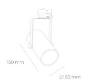
COB 3500 [K] HI EFFICIENT Light colour CRI 90 Led chip flux 3904 [lm] Luminous flux 3513 [lm] System power 25 [W] Luminaire Efficiency 141 [lm/W] Beam angle 45° Controller ON/OFF MacAdam 3 SDCM
