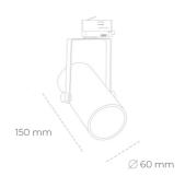
COB 4200 [K] MEAT WHITE Light colour CRI 90 Led chip flux 1412 [lm] Luminous flux 1270 [lm] System power 14 [W] Luminaire Efficiency 91 [lm/W] Beam angle 15° Controller ON/OFF MacAdam 3 SDCM
