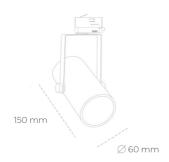
COB 4000 [K] HI EFFICIENT Light colour CRI 90 Led chip flux 4385 [lm] Luminous flux 3946 [lm] System power 27 [W] Luminaire Efficiency 146 [lm/W] Beam angle 60° Controller ON/OFF MacAdam 3 SDCM
