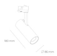
COB 4200 [K] MEAT WHITE Light colour CRI 90 Led chip flux 1976 [lm] Luminous flux 1778 [lm] System power 19 [W] Luminaire Efficiency 94 [lm/W] Beam angle 45° Controller ON/OFF MacAdam 3 SDCM
