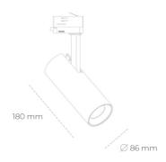
COB 4000 [K] HI EFFICIENT Light colour CRI 90 Led chip flux 3189 [lm] Luminous flux 2870 [lm] System power 19 [W] Luminaire Efficiency 151 [lm/W] Beam angle 23° Controller ON/OFF MacAdam 3 SDCM
