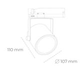
COB 4000 [K] HI EFFICIENT Light colour CRI 90 Led chip flux 4964 [lm] Luminous flux 4467 [lm] System power 31 [W] Luminaire Efficiency 144 [lm/W] Beam angle 45° Controller ON/OFF MacAdam 3 SDCM
