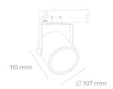
COB Light colour 2700 [K] | CRI Led chip flux 1111 [lm] Luminous flux 999 [lm] System power 10 [W] 100 [lm/W] Luminaire Efficiency Beam angle 15° Controller ON/OFF MacAdam 3 SDCM
