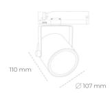
COB 3500 [K] HI EFFICIENT Light colour CRI 90 Led chip flux 3341 [lm] Luminous flux 3006 [lm] System power 21 [W] Luminaire Efficiency 143 [lm/W] Beam angle 60° Controller ON/OFF MacAdam
