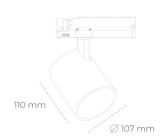
COB 3500 [K] HI EFFICIENT Light colour CRI 90 Led chip flux 3904 [lm] Luminous flux 3513 [lm] System power 25 [W] Luminaire Efficiency 141 [lm/W] Beam angle 15° Controller ON/OFF MacAdam
