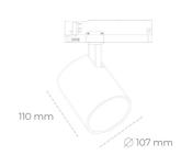
COB 3000 [K] HI EFFICIENT Light colour CRI 90 Led chip flux 1623 [lm] Luminous flux 1460 [lm] System power 10 [W] Luminaire Efficiency 146 [lm/W] Beam angle 23° Controller ON/OFF MacAdam
