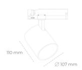
COB 3000 [K] HI EFFICIENT Light colour CRI 90 Led chip flux 3184 [lm] Luminous flux 2865 [lm] System power 19 [W] Luminaire Efficiency 151 [lm/W] Beam angle 23° Controller ON/OFF MacAdam
