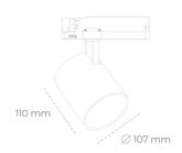
COB 3000 [K] HI EFFICIENT Light colour CRI 90 Led chip flux 3487 [lm] Luminous flux 3138 [lm] System power 21 [W] Luminaire Efficiency 149 [lm/W] Beam angle 15° Controller ON/OFF MacAdam 3 SDCM
