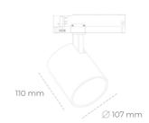
2000 [K] MEAT PINK Light colour CRI 2349 [lm] Led chip flux Luminous flux 2114 [lm] System power 27 [W] Luminaire Efficiency 78 [lm/W]
