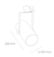
COB 3000 [K] HI EFFICIENT Light colour CRI 90 Led chip flux 4378 [lm] Luminous flux 3940 [lm] System power 27 [W] Luminaire Efficiency 146 [lm/W] Beam angle 38° Controller ON/OFF MacAdam 3 SDCM
