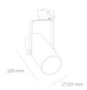
COB 3500 [K] HI EFFICIENT Light colour CRI 90 Led chip flux 3054 [lm] Luminous flux 2748 [lm] System power 19 [W] Luminaire Efficiency 145 [lm/W] Beam angle 15° Controller ON/OFF MacAdam 3 SDCM
