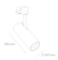
COB 3500 [K] HI EFFICIENT Light colour CRI 90 Led chip flux 2174 [lm] Luminous flux 1956 [lm] System power 14 [W] Luminaire Efficiency 140 [lm/W] Beam angle 60° Controller ON/OFF MacAdam 3 SDCM
