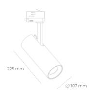
COB 3500 [K] HI EFFICIENT Light colour CRI 90 Led chip flux 4723 [lm] Luminous flux 4250 [lm] System power 31 [W] Luminaire Efficiency 137 [lm/W] Beam angle 38° Controller ON/OFF MacAdam 3 SDCM
