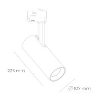
COB 2000 [K] MEAT PINK Light colour CRI 1845 [lm] Led chip flux Luminous flux 1660 [lm] System power 21 [W] Luminaire Efficiency 79 [lm/W] Beam angle 38° Controller ON/OFF
