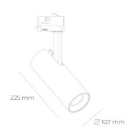
COB Light colour 2700 [K] | CRI 2888 [lm] Led chip flux Luminous flux 2599 [lm] System power 25 [W] Luminaire Efficiency 104 [lm/W] Beam angle 23° Controller ON/OFF MacAdam 3 SDCM
